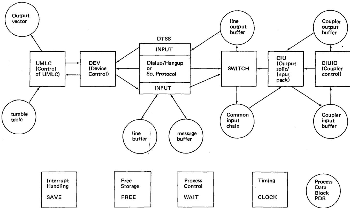
Fig. 7.1 – Simplified software structure.
