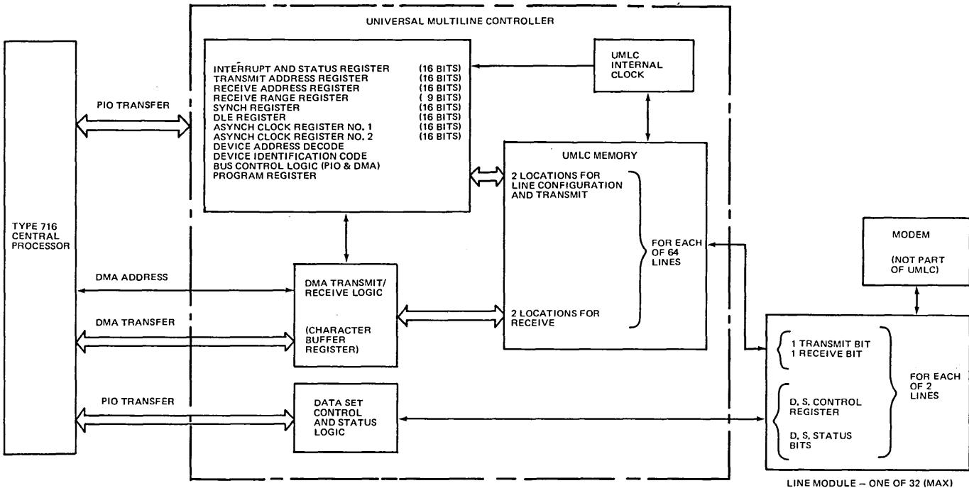
Fig. 7.5 – Block diagram of UMLC.
