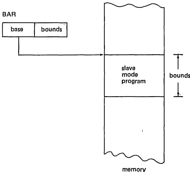
Fig. 2.3 – Base address register.
